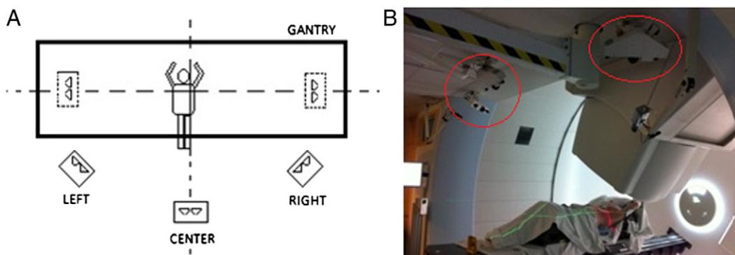
**Figure 1** **(A)** AlignRT camera positions in the proton gantry room. The thicker line box marks the location of the rotating gantry structure. As a result, the 2 side cameras must be moved to outside of the gantry rotation area, instead of the location indicated by the dashed line boxes, as in a typical LINAC room installation. **(B)** Actual system in place at Massachusetts General Hospital.
