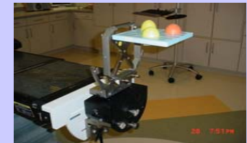
Figure 3. A view of the bite block assembly when attached to the Leksell frame and couch mount manipulator.
